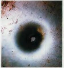
Polev sub-caliber 511.5-grain lead slug fired at a distance of 55 yards blew through 0.08-inch steel plate.
